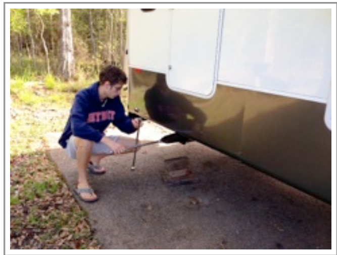
Harrison uses a 4-way wrench to lower the rear scissors jacks.
