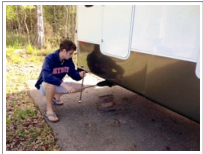
Harrison uses a 4-way wrench to lower the rear scissors jacks.
